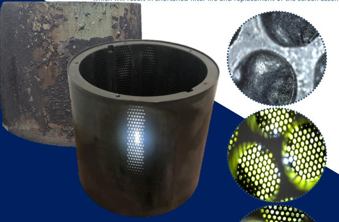
Microscopic inspection of the conical and internal screen structure during and after cleaning provides essential information about the degree of cleanliness of the Ettlinger Screen assembly prior to installation.
